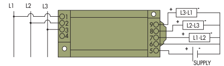
CR4860 3 Element, 3 Wire - 4-20 mA DC Output
